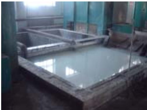
Cooling Pool for Heat Treatment
