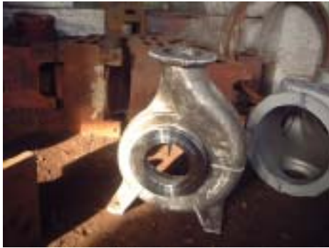
S.S. Chemical Pumps
